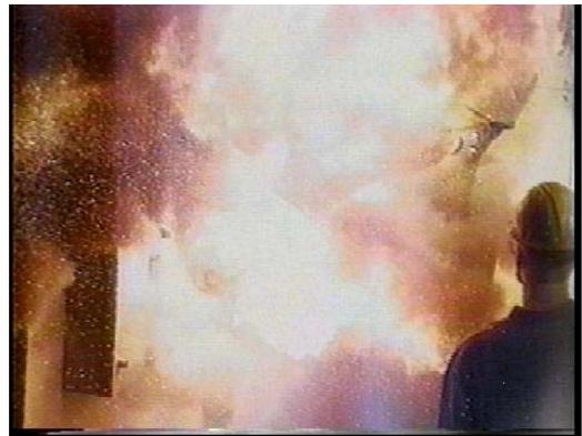
The question that remains is how can these hazards be limited? Several design concepts are available that can limit these electrical hazards. One possible solution is the use of current-limiting devices. Current-limiting devices have the ability to greatly reduce the electrical hazards from high level arcing faults. In addition, “finger-safe” devices can be added to reduce the possibility of contact with live parts.
