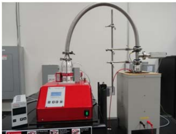
Figure 9: Test Setup for Developing Vacuum Versus Current Flow Data
