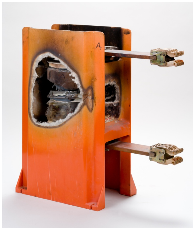
Figure 5: Failed Vacuum Interrupter
