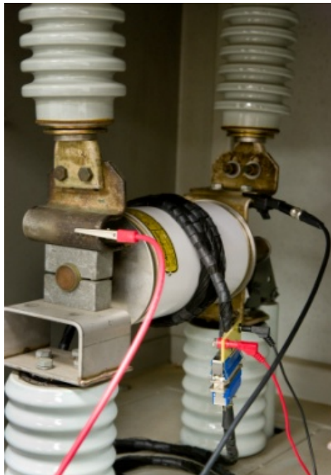
Figure 7: Flexible Magnetic Field Coils
